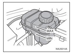
The engine coolant surge tank is located in the rear of the engine compartment on the driver's side.
